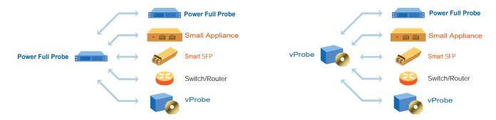
All types of Probes (Hardware or Software) acts as TWAMP Initiator & Reflector. Only Smat SFP act as Reflector Only with TWAMP light.
